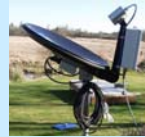
MRR observes a profile of the atmosphere
