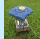
JW disdrometer collects precise rainrate data
