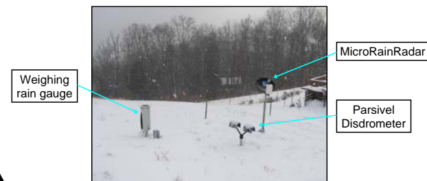
Figure 3: Precipitation instruments during a heavy snow event
