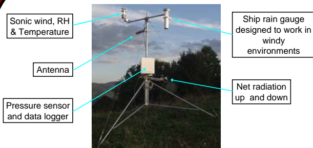
Figure 2: Meteorological tower on the top of Poga Mountain
