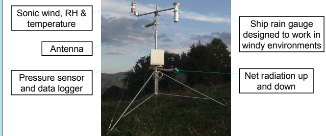
Figure 1: Meteorological tower on the top of Poga Mountain
