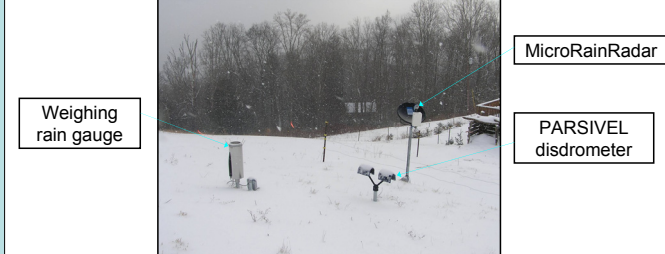
Figure 2: Precipitation instruments during a light snow event
