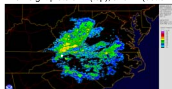
Figure 3: Horizontal radar scan at 00:16 UTC from WSR-88D NEXRAD located at Roanoke, VA (KFCX). The radar beam is blocked near Poga Mountain so precipitation echoes will be underestimated. White marker indicates the location of the MRR at Poga Mountain, NC
