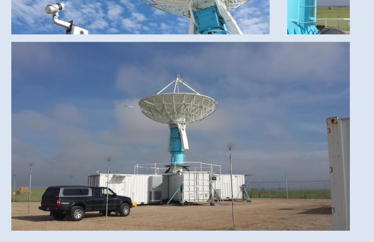
Two radars were remotely controlled from Dr. Yuter's laboratory at North Carolina State University. SPol, located in Firestone, CO, is owned by the National Center for Atmospheric Research (NCAR). It sits atop storage containers which can be packed up and shipped all over the world. CHILL, located in Greeley, CO, is owned by Colorado State University and is housed in an air-supported dome to protect it from the elements.
