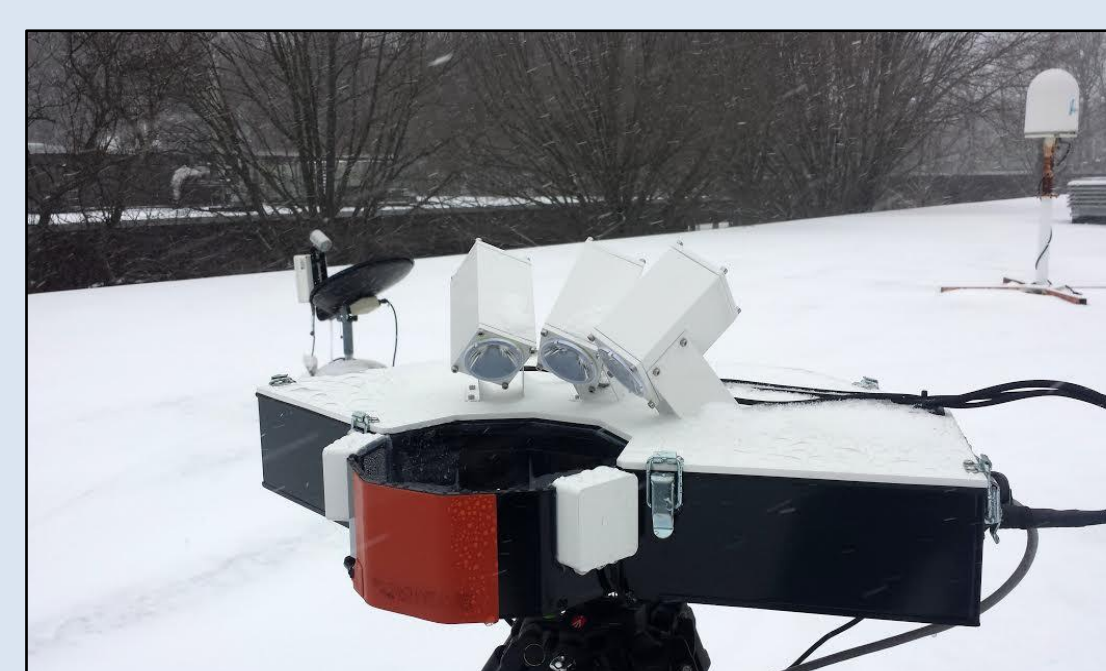
Multi-Angle Snowflake Camera (foreground) and vertical radar (background) at Stony Brook University during winter 2014-15
