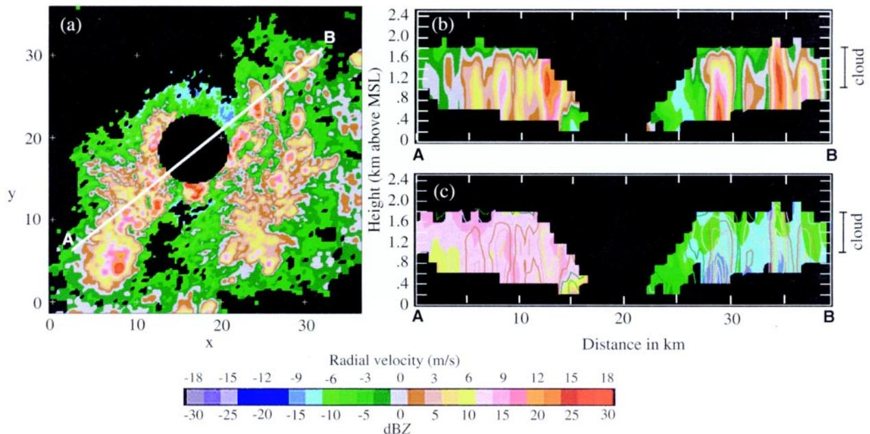
FIG. 8. Ship-based C-band radar data within the marine stratocumulus region. Interpolated three-dimensional volume data from 1035 UTC 2 Sep 1997. (a) Horizontal cross section of radar reflectivity at 1-km altitude, (b) vertical cross section of radar reflectivity along line A–B in (a), and (c) vertical cross section of radial velocity along line A–B in (a) with radar reflectivity contours overlain. Reflectivity contours, color bar, and interpolated volume resolution as in Fig. 7.
