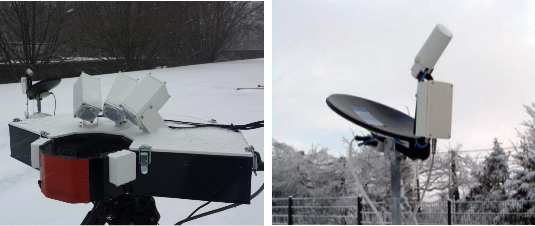
Figure 1. Multi Angle Snowflake Camera (MASC)
