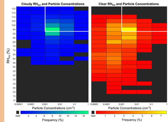
2D histograms plotting frequencies of concurrent 100-m horizontal scale RH<sub>ice</sub> and 2D-S concentration data (100-2000 μm diameter) during 21 cloud sandwich legs. The data from the legs were divided into times that were visually cloudy and clear using the P-3 video observations. The white lines outline the region of RH<sub>ice</sub> ≥ 95% and 2D-S concentrations ≥ 0.001 cm<sup>-3</sup>.
