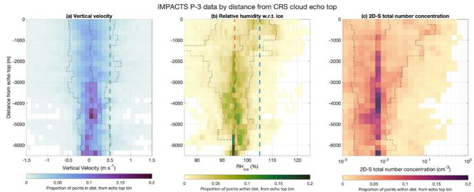
2D histograms depicting 100-m horizontal scale (a) in situ vertical velocity, (b) RH<sub>ice</sub>, and (c) 2D-S particle concentration relative to distance from cloud echo tops from IMPACTS data (Allen et al, 2025).
